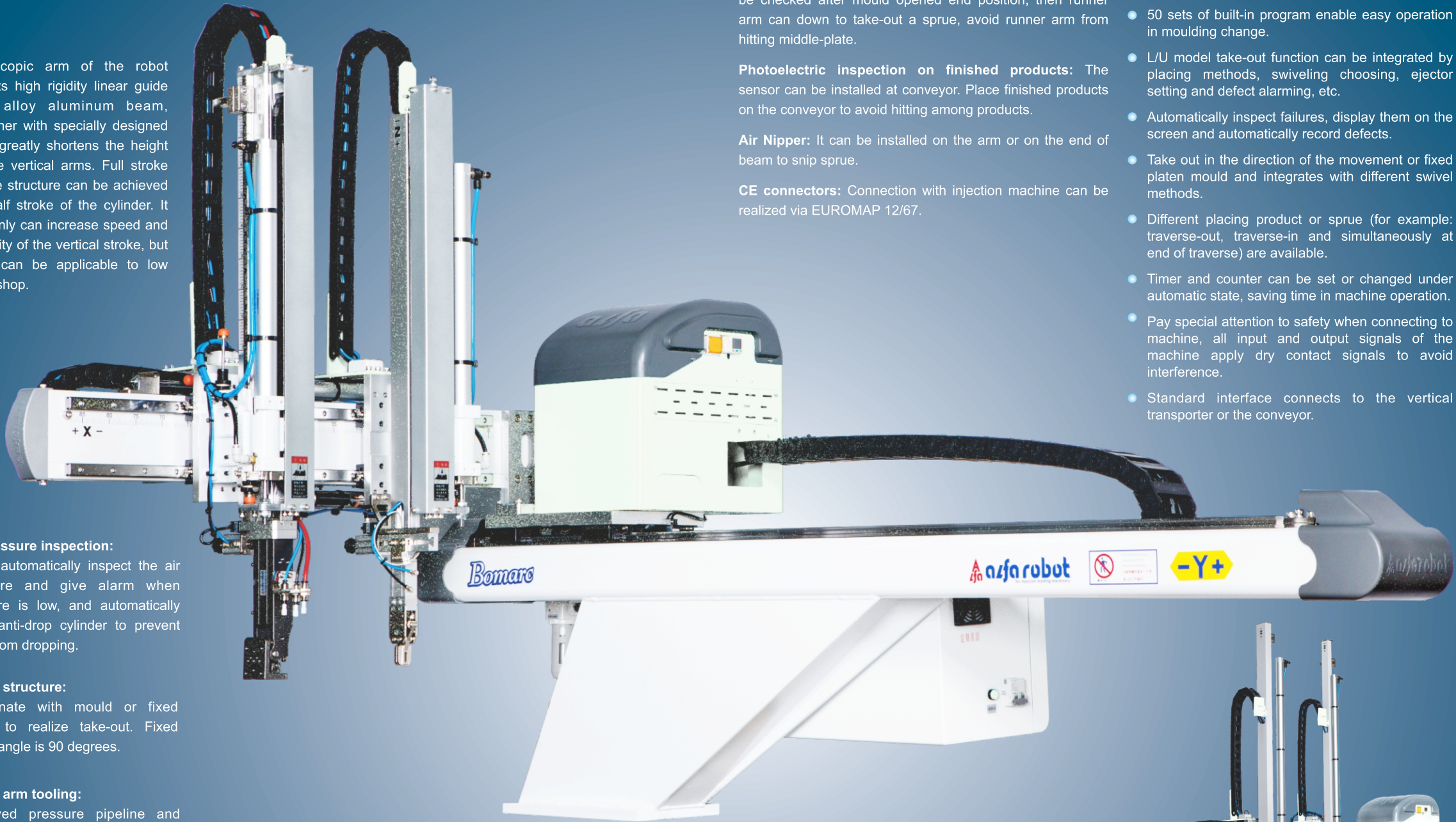
BE850WDY Telescopic/ Double arms/ Traverse driven by AC servo motor
